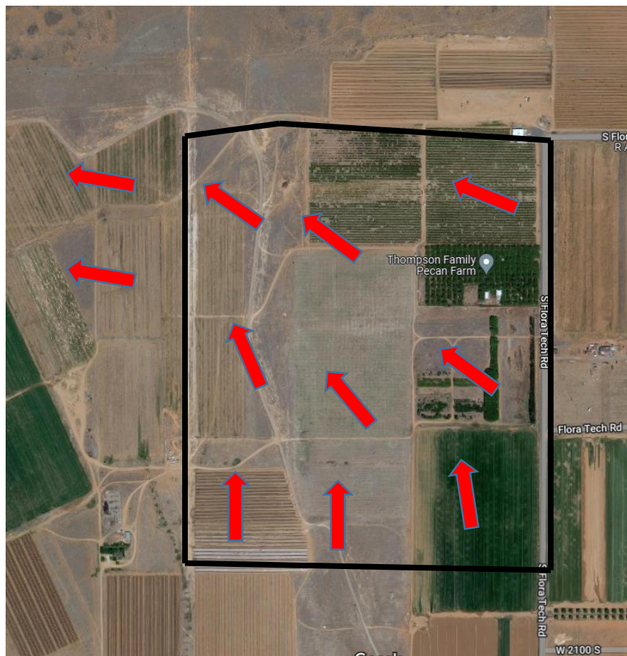
Figure 2.1.1: Existing Drainage Condition
