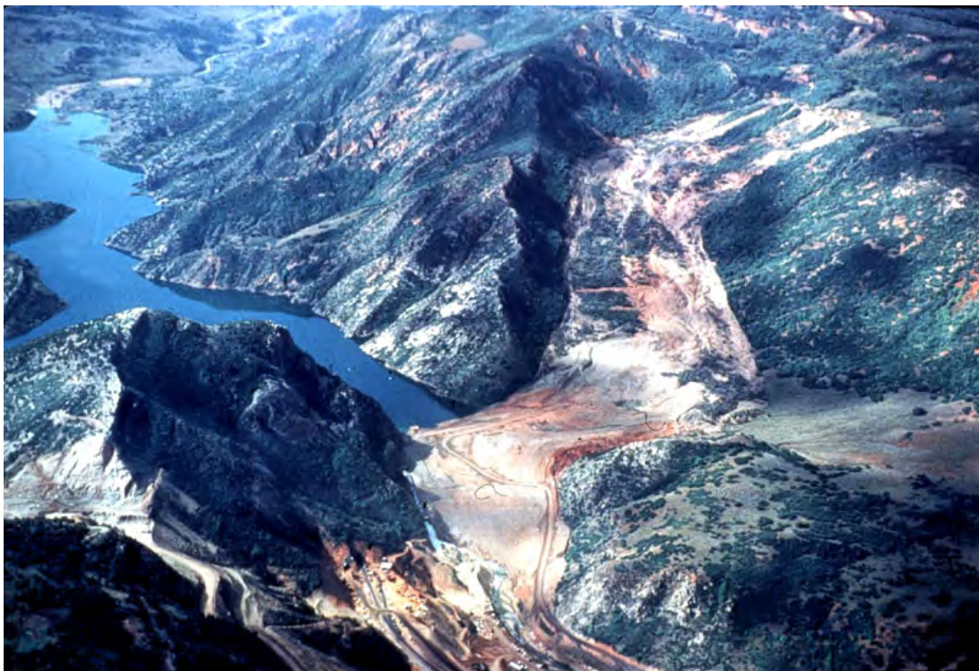
Figure 22. The 1983 Thistle, Utah, landslide buried parts of two State highways and the Denver and Rio Grande Railroad. The landslide also dammed two streams, resulting in a 3-mile-long and 200-foot-deep lake that inundated the town of Thistle and posed a flooding hazard to communities downstream. Aerial photograph provided by the USGS National Landslide Information Center.
