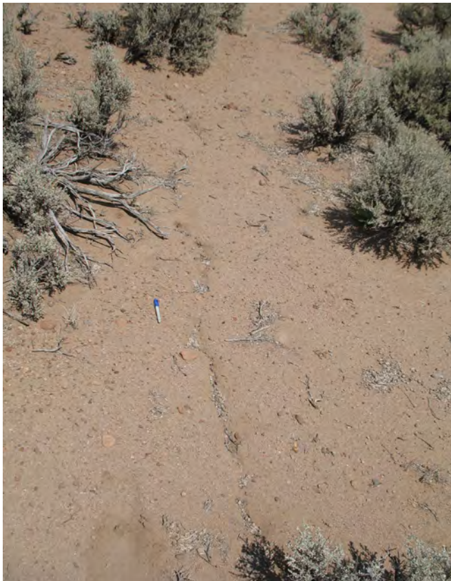
Figure 31. Earth fissure in Cedar Valley expressed as an uneroded primary ground crack. This fissure could be traced for 900 feet before becoming obscured by recent agricultural activity. Photo taken in August 2009.
