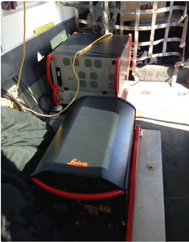
Figure C5. Leica ALS70 lidar instrument mounted in a Piper Navajo aircraft used for the 2013 Utah acquisition by the Utah Geological Survey and partners (photo credit: Watershed Sciences, Inc.)
