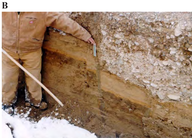
Figure 8. Normal fault: (A) schematic diagram, (B) exposed in an excavation (photo courtesy of David Simon).
