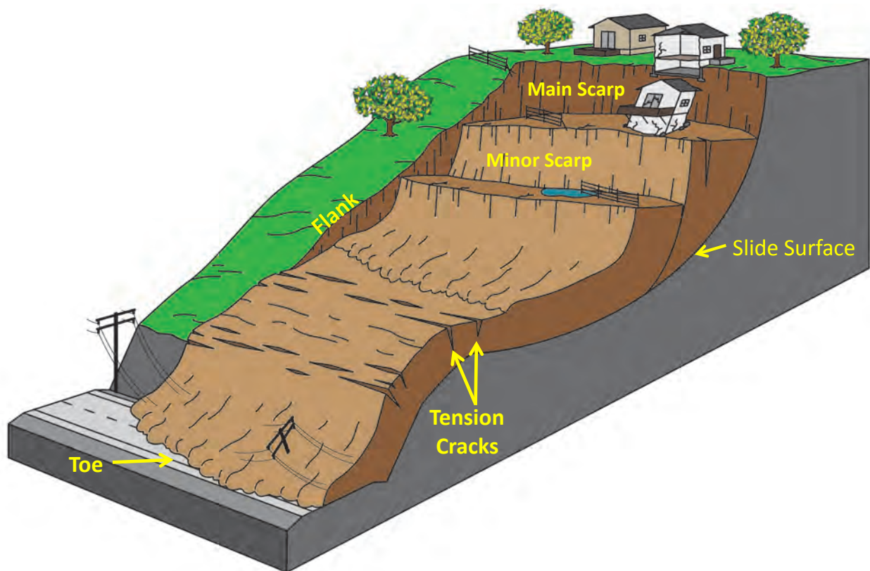
Figure 21. Diagram of an idealized landslide showing commonly used nomenclature for its parts.
