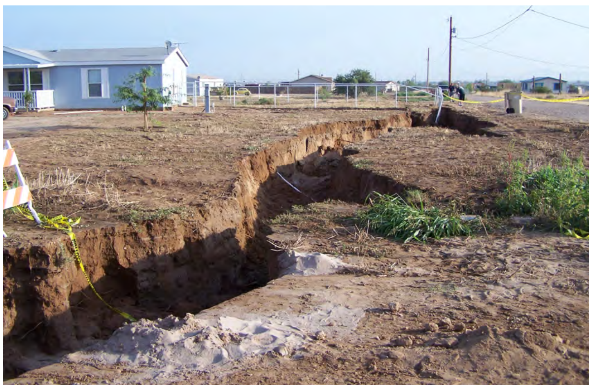
Figure 36. Earth fissure in a subdivision near Phoenix, Arizona, enhanced by erosion during a cloudburst storm. Photo credit: Brian Conway.
