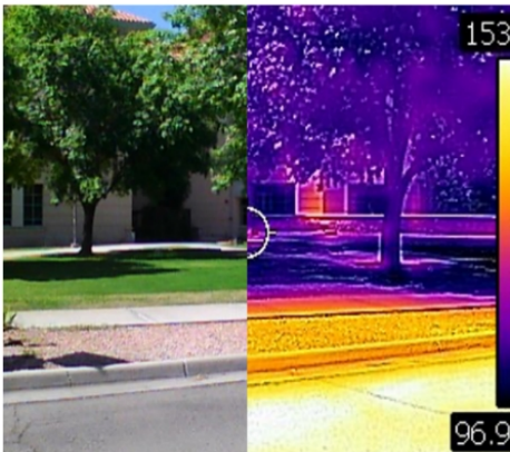
Figure 2.15. Thermal image (right) taken in Las Cruces, New Mexico, showing hotter areas in brighter colors with cooler areas in darker colors, with temperatures displayed in Fahrenheit (Dave DuBois/U.S. NOAA)
